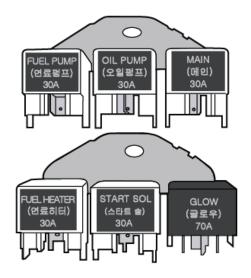
Using an ohmmeter, check that there is continuity between each terminal.
