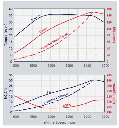
\*BSFC : Brake Specific Fuel Consumption \*FC : Fuel Consumption
