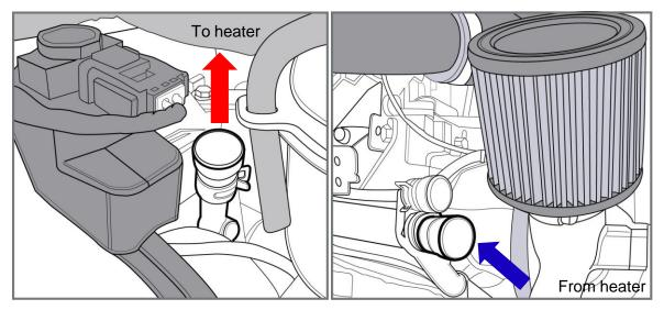
\* Outer diameter of line is Ø19.3 mm
