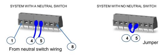
2) If there is a dual EOI, you should connect the wiring between #5 (external connector of the main EOI) and #5 (external connector of the dual EOI)
